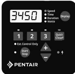
Figure 12: Setting Speed for Quick Clean
