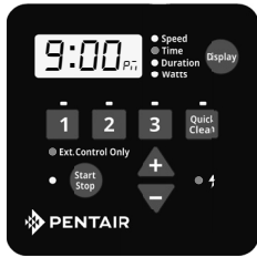
Figure 7: Activating External Control Only
