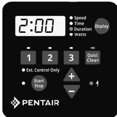
Figure 13: Setting Duration for Quick Clean
